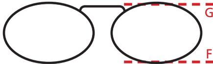
! For rimless frames, adjust boundaries to the front face of the lens, where the lens ends.
