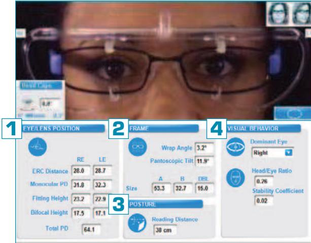
5 For Essilor personalized designs requiring the Natural Head Posture measurement, manually set your patient’s head rotation (**Head Cape**) to the non-zero value. The measurement results will be adjusted automatically.
