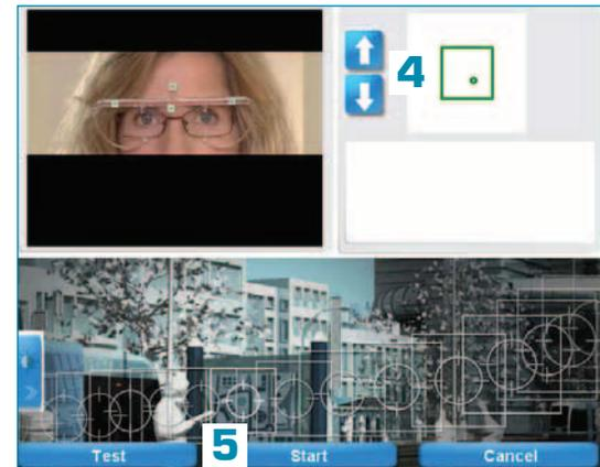
5 Press the Start button to begin recording. While measurements are acquiring, the progress of the 25 trackings will be displayed on the screen.
